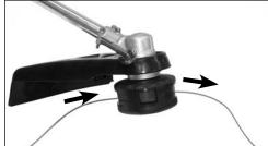
4. Hold trimmer head while turning knob clockwise to wind line onto spool until about 5" (13 cm) of each line remains exposed.
